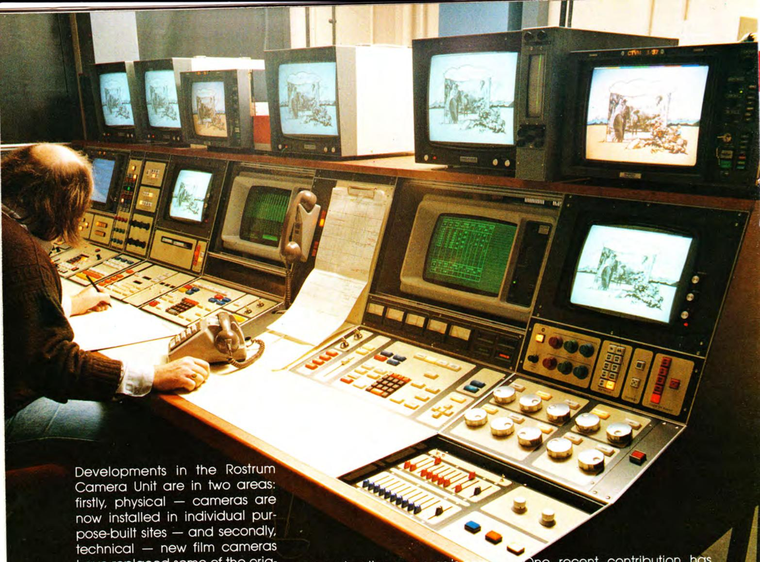
Developments in the Rostrum Camera Unit are in two areas: firstly, physical — cameras are now installed in individual purpose-built sites — and secondly, technical — new film cameras have replaced some of the originals, and the completion of the video rostrum camera has added greater flexibility to the unit as a whole.
